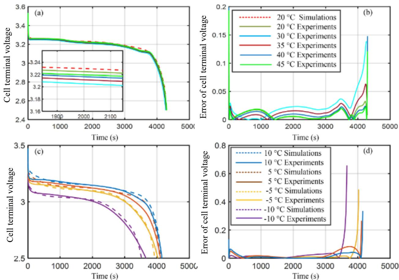
**Simulations of terminal voltage and errors for cell B3**
