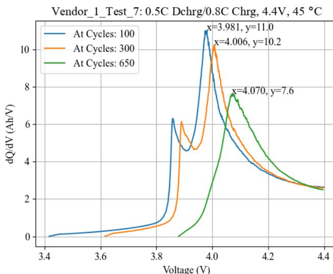
**Figure 2. Evolution of battery Differential Capacity curve with cycling.**
