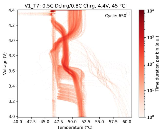
**Figure 1. Battery Voltage-Temperature colormap as stress factors.**
