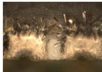
**Silver Sulfide Formation of Chip Resistor**
